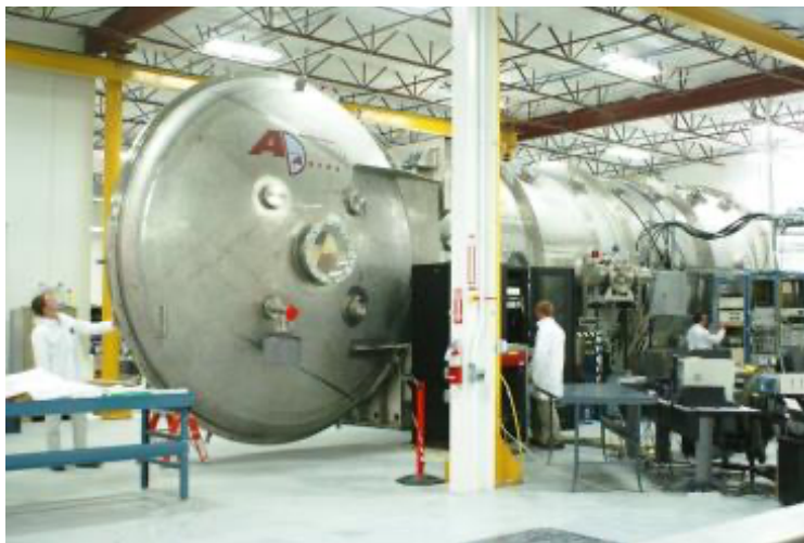
150 m 3 , < 10 -8 torr base pressure Large Space Simulation Chamber. Source: Ad Astra Rocket Company
